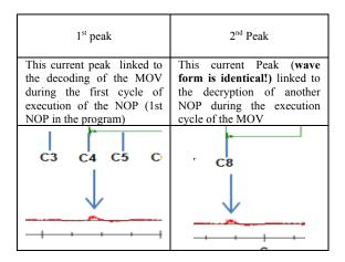
Analysis of the above trace, and highlighting of the influence of the pipeline on consumption
