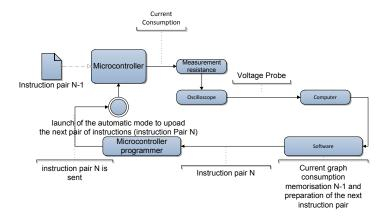
In the follow up of this analysis, for more simplicity<sup>5</sup>, we will only look into instructions which last just one machine cycle. If, as a minimum, we want to find all the possible pairs of two instructions with the matching data, we need 256<sup>2</sup> or 65536 measurements
