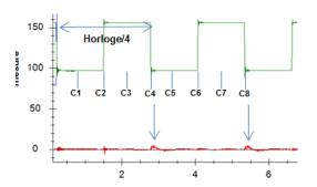
C1, C2..., C8: represents the steps for decoding an instruction on a PIC: An instruction is executed every four clock cycles on this type of microcontroller. Each cycle corresponds to specific decoding step (this is the pipeline!) . In comparison to the program 2 (nop, movlw 0x00, nop, nop), this is how the instructions are dealt with on the pipeline
