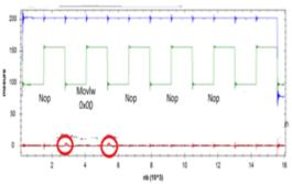
In red trace above, the 2 circled small current's peaks represent the consumption which is theoretically proportional to the number of bits transitions which are going from 1 to 0 or from 0 to 1: in our case, it's correspond to the number of bits of nop and a movlw instructions.
