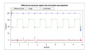
In relation to the second program (which contained a movlw 0X00), we can see a difference in measurements linked to the difference in the number of 0 bits and 1 bits between the two instructions
